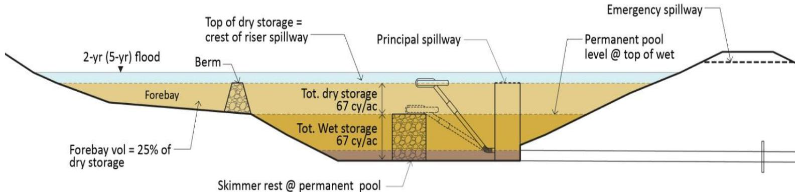
Temporary sediment basin formed by an embankment dam and showing various features, including wet and dry storage volume components, forebay cell, surface water skimmer, and separate principal and emergency spillways (Note: 25-yr flood level and spillway design freeboard distances not shown).
